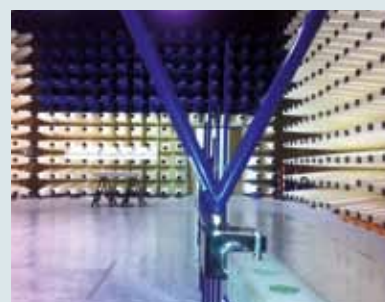
New 10m range Semi Anechoic chamber at CEI – accredited by INAB to perform radio frequency emissions testing.
